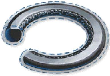
**Contributing Factors:** Improper or improperly cured elastomer. High vacuum levels. Low hardness/plasticized elastomer.
