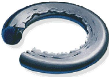
**Contributing Factors:** Excessive clearances. Excessive pressure. Low-modulus/hardness elastomer. Excessive gland fill. Irregular clearance gaps. Sharp gland edges. Improper sizing.
