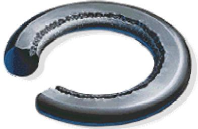
**Contributing Factors:** Chemical reactivity of the plasma. Ion bombardment (sputtering). Electron bombardment (heating). Improper gland design. Incompatible seal material.
