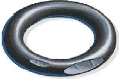
**Contributing Factors:** Sharp edges on glands or components. Improper sizing of elastomer. Low-modulus/hardness elastomer. Elastomer surface contamination.
