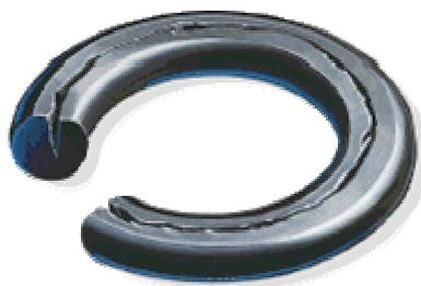
**Contributing Factors:** Improper design—failure to account for thermal or chemical volume changes, or excessive compression.
