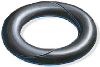
**Contributing Factors:** Difficult or tight installation (static). Slow reciprocating speed. Low-modulus/hardness elastomer. Irregular O-ring surface finish (including excessive parting line). Excessive gland width. Irregular or rough gland surface finish. Inadequate lubrication.
