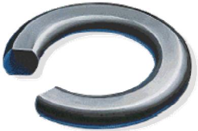
**Contributing Factors:** Excessive compression. Excessive temperature. Incompletely cured elastomer. Elastomer with high compression set. Excessive volume swell in chemical.
