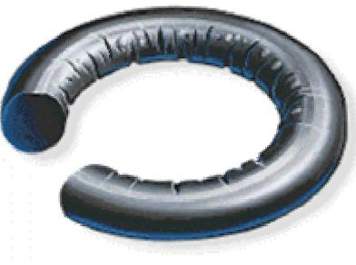
**Contributing Factors:** Elastomer thermal properties. Excessive temperature excursions or cycling.
