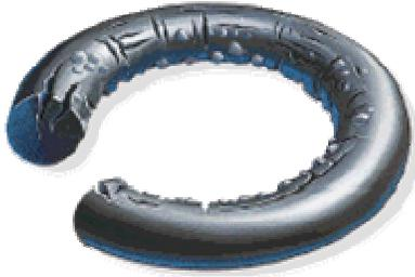
**Contributing Factors:** Rapid pressure changes. Low-modulus/hardness elastomer.
